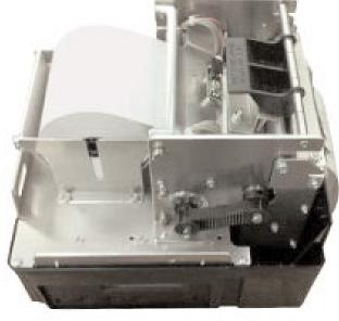
**Power Requirements** 100-240 VAC, 50/60 Hz, 80W max 24 V DC, 100W max
